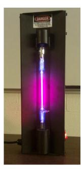
The pinkish glow of a Hydrogen discharge lamp is a mixture of colors and wavelengths. Watch the Panopto video.
