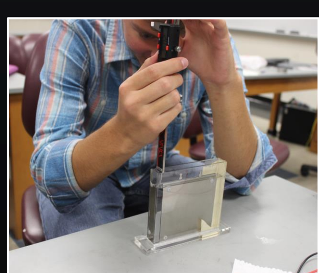
Using a depth-measuring probe to measure the height of the oil
